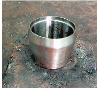
A hardened steel turned cutting tip
