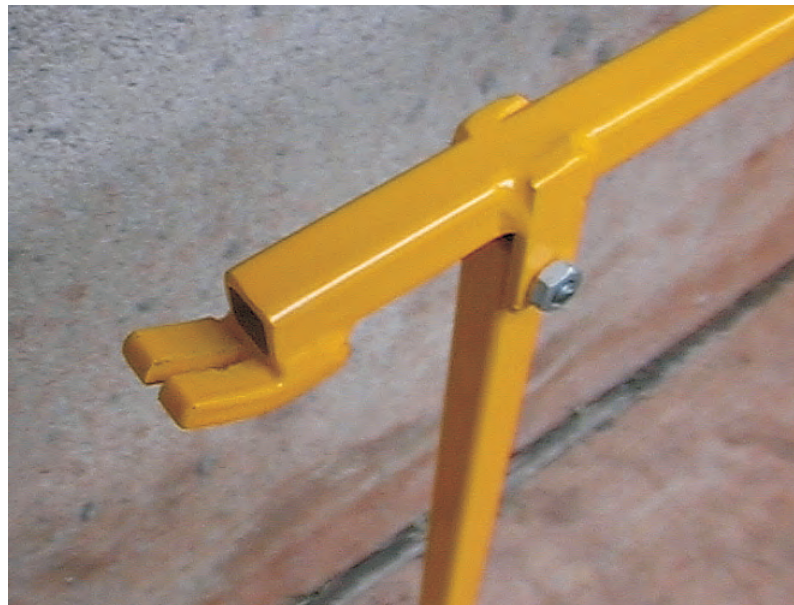
Claw for pulling chain on jack lever
