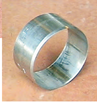
Close-up view of thin-walled soil sampling ring
