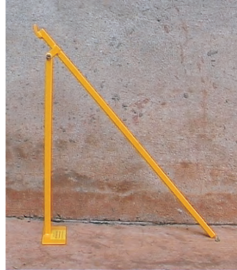
Hand-jack for extracting core tube
