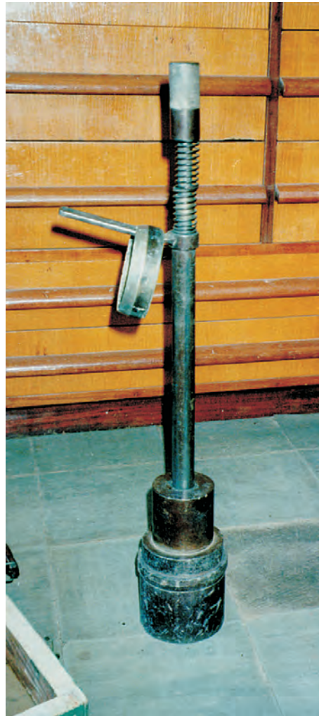
A sliding hammer for sampling bulk density. The removable cutting tip is placed onto the end of a removable steel ring which is inserted into the body of the sampler. After sampling, the cutting tip is removed and the ring sealed for later processing of the sample.
