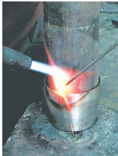
Silver solder the turned tip onto the tube.
