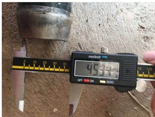
Photo 3 Measuring the internal cutting diameter of the soil coring tube using callipers
