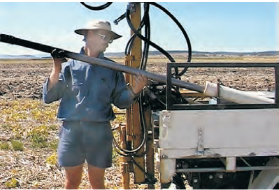
A pull-through made of an oily rag attached to a weight with a rope will lubricate the inside of the tube without leaving excess oil.
