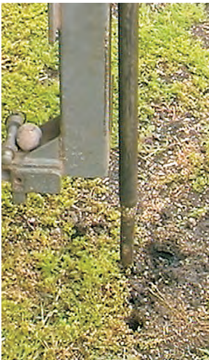
A core sliding back into the core hole as the tube is removed from the soil .
