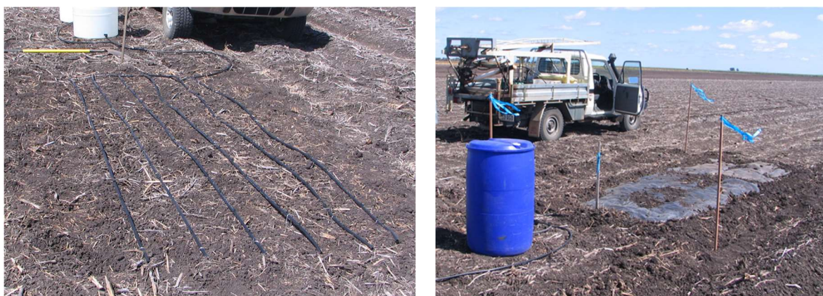
Photo 1 A dripper array system placed over the soil surface to wet up a covered plot
