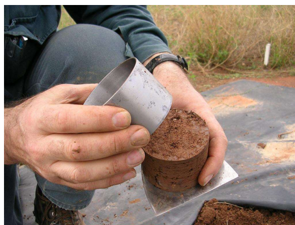
Photo 7 BD ring used to collect a known volume of soil
