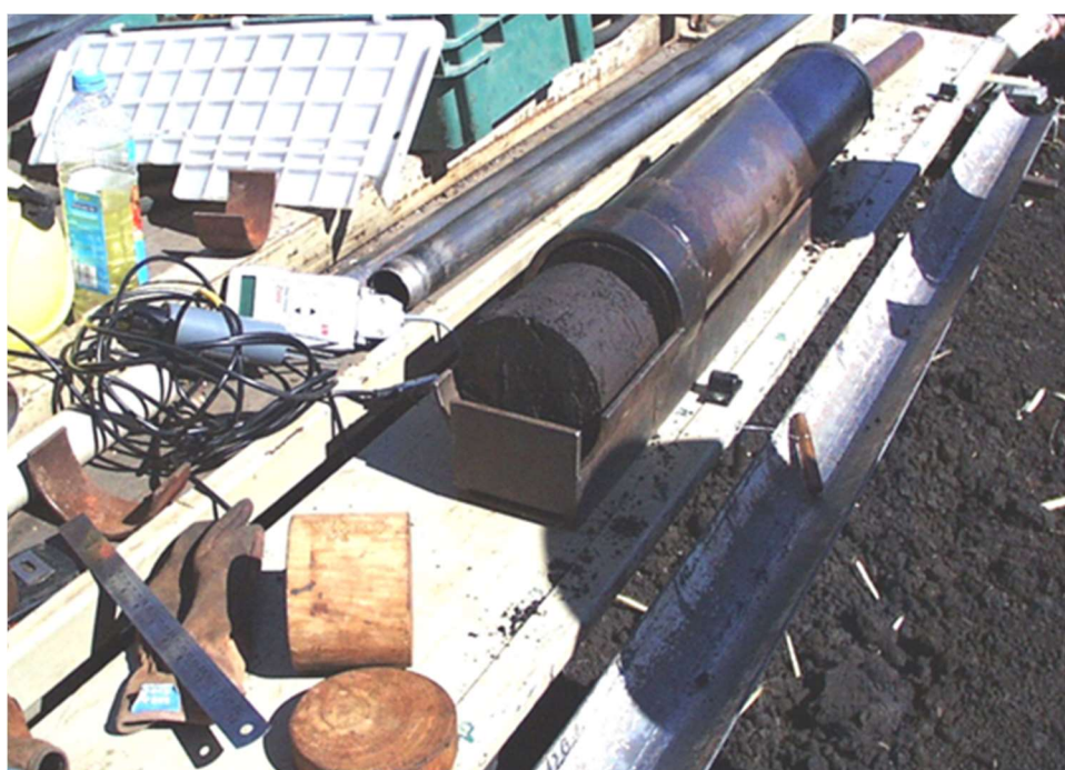
Photo 8 Large diameter soil coring apparatus used to take BD measurements
