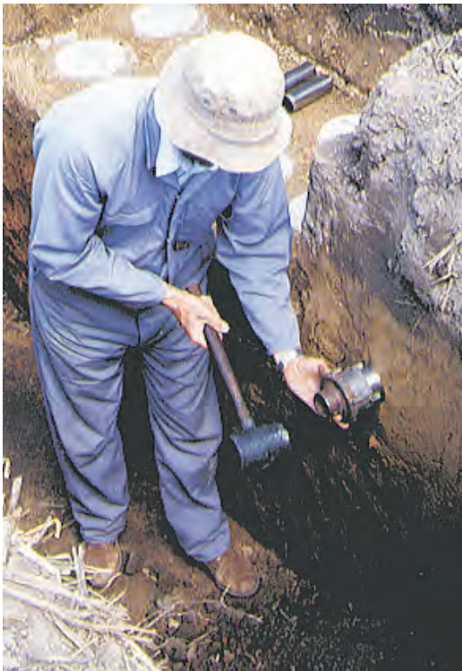
Measuring bulk density: driving a sampling ring into the wall of a pit (Photo B. Bridge)
