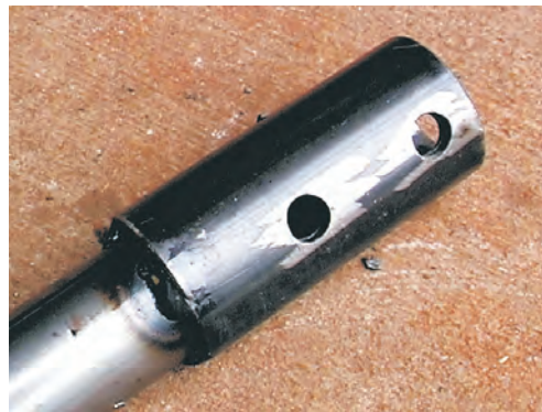
The tube collar with holes for extraction pin and spot-welds around its lower edge.
