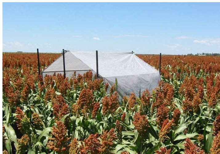
Photo 2 Rainout cover placed over a sorghum crop to stress the crop to wilting point
