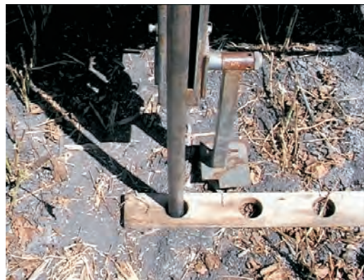
A core-locating board ensures that a set of samples is taken in pre-determined locations relative to the row.
