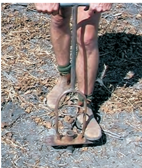
A stirrup sampler—a useful tool for surface sampling for P and Zn.
