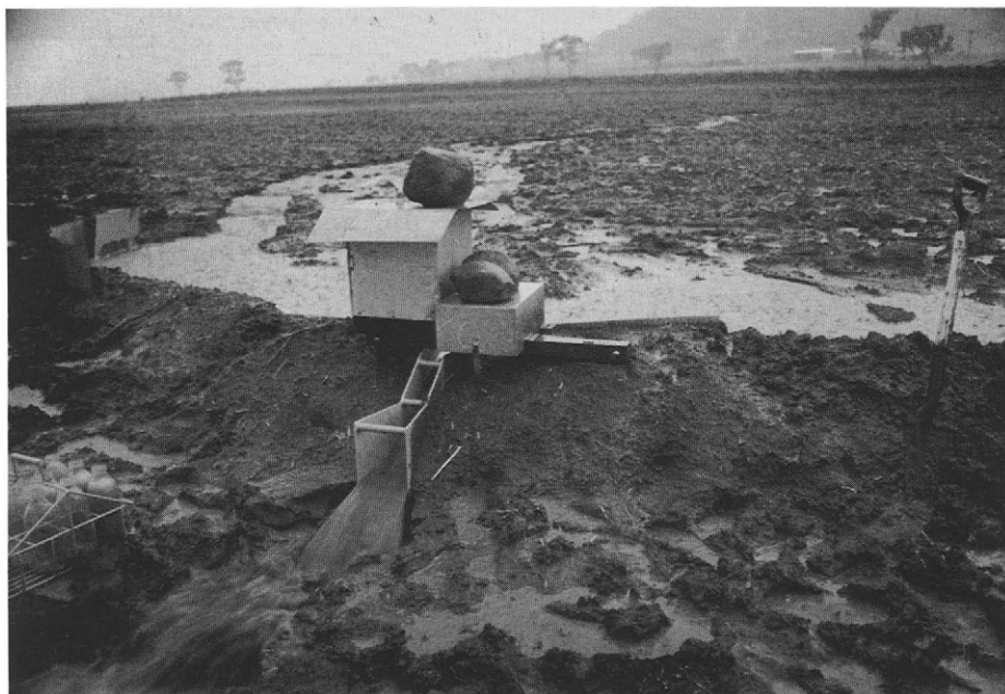
Fig. 9.18. "Rill" catchment instrumented to measure runoff and sample water.
