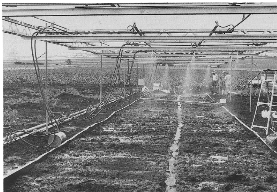
Fig. 9.16. Photograph of the "Rainulator" used to study erosion processes. The plot area is 22 \times 4 m and rainfall can be applied at up to 100 \text{ mm hr}^{-1} (McKay and Loch, 1978).
