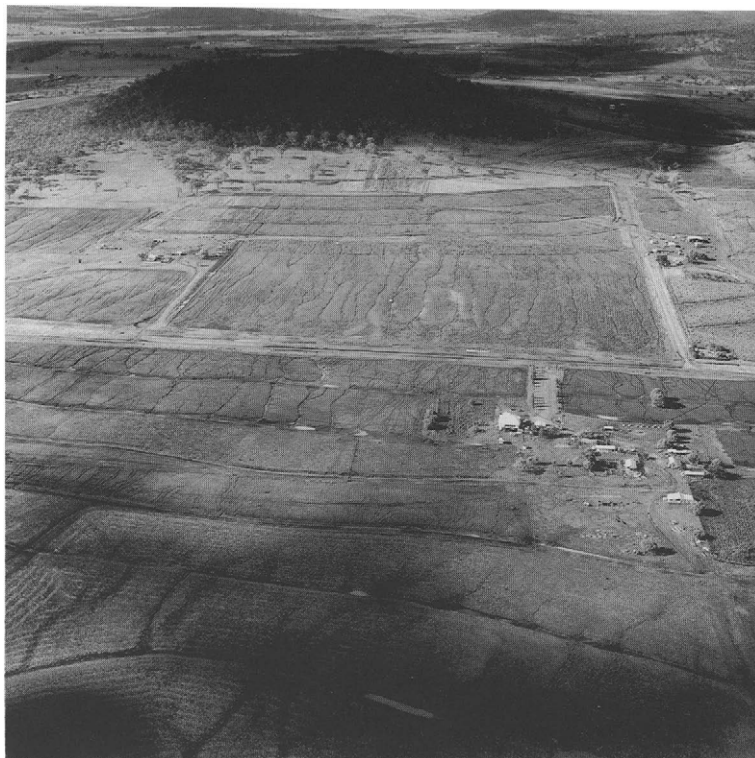
Fig. 9.17. Typical patterns of water flow and erosion on basalt derived vertisols in north eastern Australia. Once rilling occurs, subsequent rills develop in the same area reinforcing a fixed pattern of erosion.
