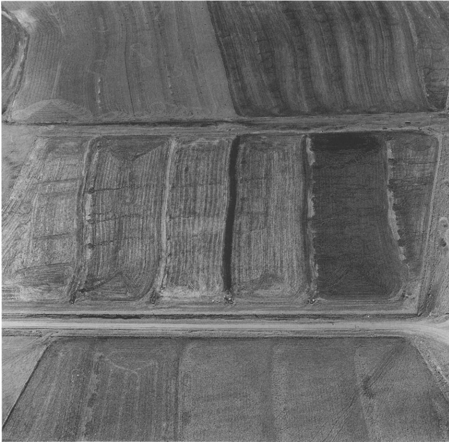
Fig. 9.19. Oblique aerial photograph of a field study showing five instrumented catchments. Different management options can be implemented in each catchment which represents the smallest management hydrologic unit in many agricultural areas. Distance across photograph is approximately 350 m.
