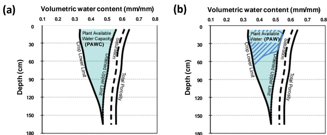
**Figure 1-1. (a) The Plant Available Water Capacity (PAWC) is the total amount of water that a soil can store and release to different crops and is defined by its Drained Upper Limit (DUL) and its crop specific Crop Lower Limit (CLL); (b) Plant Available Water (PAW) represents the volume of water stored within the soil available to the plant at a point in time. It is defined by the difference between the current volumetric soil water content and the CLL.**
