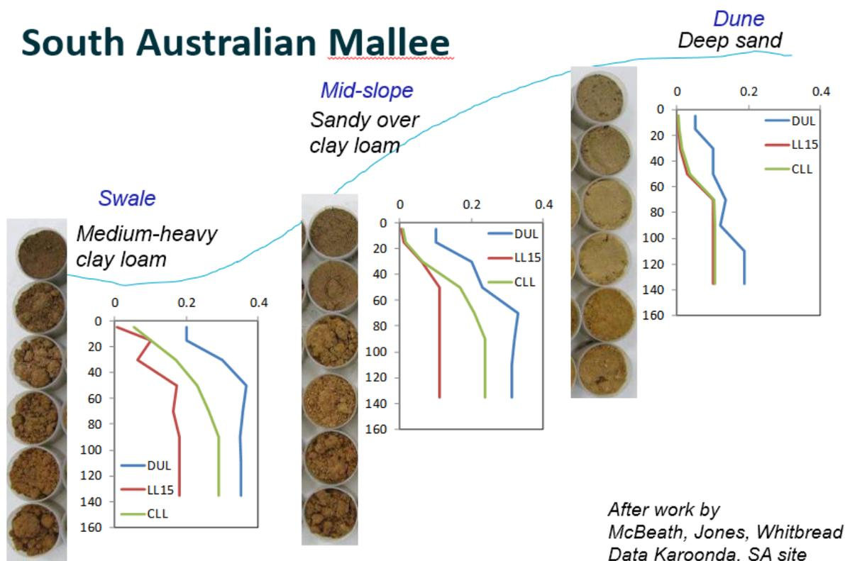
Figure 9-2. A conceptual frame-work for PAWC distribution in South Australian Mallee soils. Source: presentation by McBeath, Jones and Whitbread - Karoonda SA
