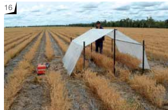
Photo 16: Rain-exclusion tent in chickpeas just prior to final sampling for CLL. Note the higher pitch on the roof to better shed water.
