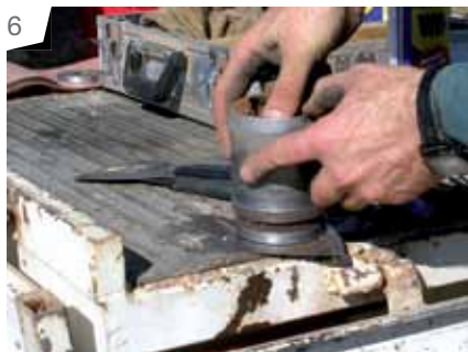
Photo 6: Disassemble the sampler body and carefully remove the sample in its rings, taking care not to damage soil core in the main ring.
