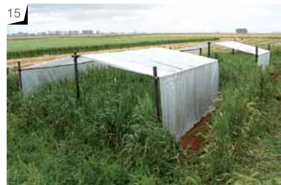
Photo 15: Rain-exclusion tent in place. Duct tape on the pipes prevents chaffing. The plastic cover lies between the posts to simplify the attachment of the tubes. At the minimum 20° pitch, the cover must be tight to shed water.
