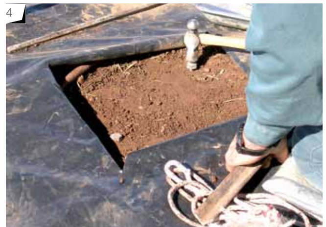
Photo 4: Locate steel datum pins either side of core site.
