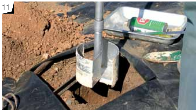
Photo 11: Removing dross and levelling the base of the auger hole in preparation for sampling (using special levelling tool).
