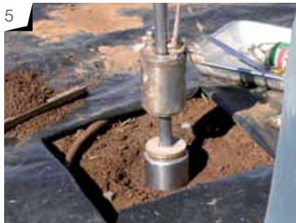
Photo 5: Auger to the first sampling point so that the sample will straddle the mid-point of the first layer. Check depth against datum pins. Lightly oil sampling rings, ensure there is no grit on the outside of the rings, assemble the BD sampler body and take the first sample.
