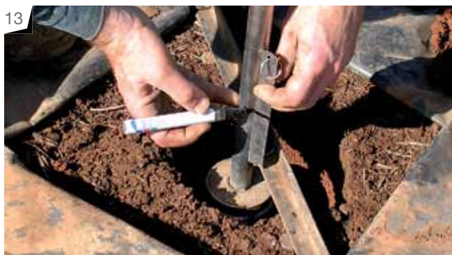
Photo 13: Referencing sampling depth. The sampler is placed in the hole and the depth of the core sample measured and marked on the shaft of the sampler using the datum pins as reference. The corer is driven into the soil until the mark reaches the line of the datum pins. Driving the sampler past the reference line will result in compaction of the sample within the corer head.
