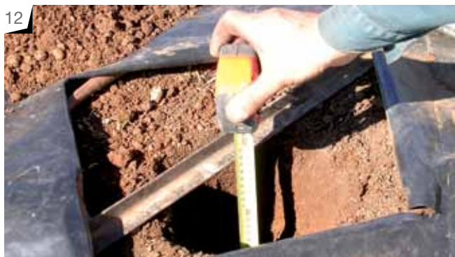
Photo 12: Checking the depth of the hole prior to sampling. All measurements are referenced to the datum pins.
