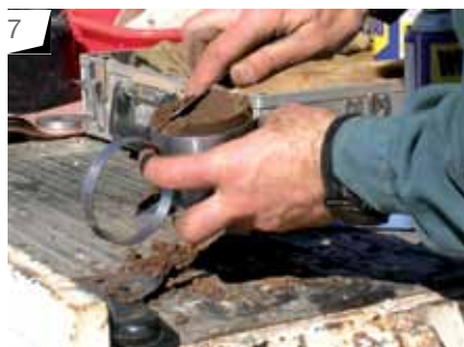
Photo 7: Remove one of the steel spacer rings and, using a knife, carefully pare back the soil level with the end of the main sampling ring; then repeat the process with the other spacer ring.
