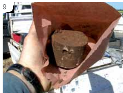
Photo 9: Slide sample from ring into storage bag. Weigh immediately if using a paper bag for DUL sampling. If using a plastic bag the sample may be weighed on return to base but the bag needs to be well sealed and stored in a cool environment.
